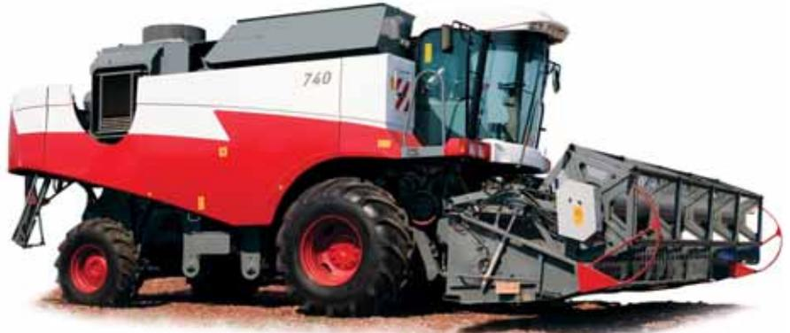
A combine harvester is a machine that harvests grain. It combines reaping, binding, and threshing into one operation. The straw left behind is either chopped and spread on the field or baled for feed and bedding for livestock.
