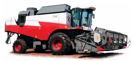
A combine harvester is a machine that harvests grain. It combines reaping, binding, and threshing into one operation. The straw left behind is either chopped and spread on the field or baled for feed and bedding for livestock.
